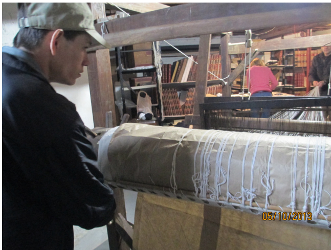
Jim Merritt at the loom, lashing the warp to the back roller and adding paper to separate the warp as new layers are rolled on.
